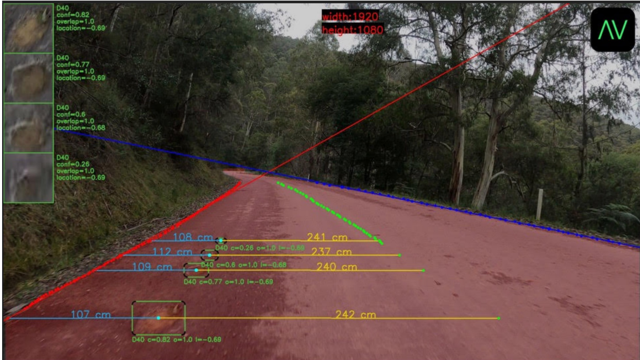
Asset Vision's AutoPilot technology detects and measures road pavement defects, along with their relative position on the road.
